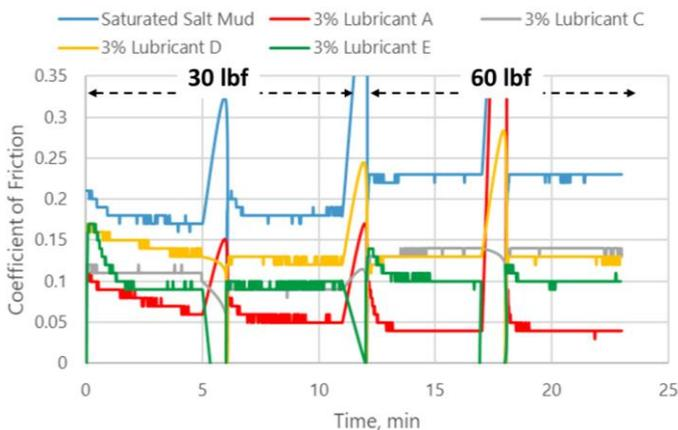
Figure 7: Lubricity of 14.0 ppg saturated salt mud on steel-steel contact measured with the LEM.
