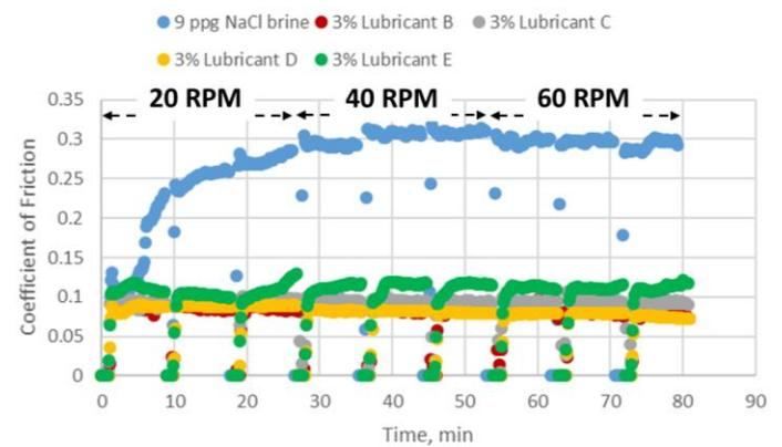
Figure 1: Lubricity of 9.0 ppg NaCl brine on steel-steel contact measured with the dynamic lubricity tester.
