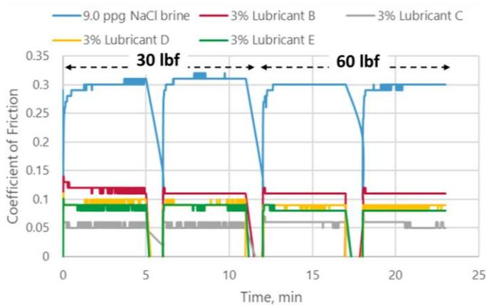
Figure 3: Lubricity of 9 ppg NaCl brine on steel-steel contact measured with the LEM.
