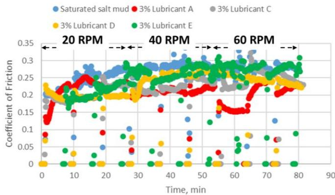
Figure 6: Lubricity of 14.0 ppg saturated salt mud on steel-shale contact measured with the dynamic lubricity tester.
