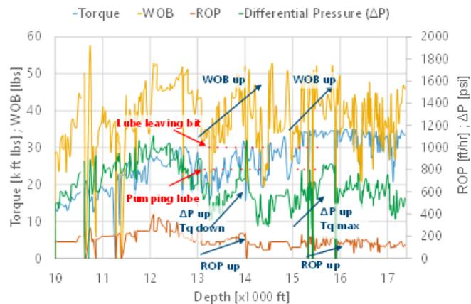
Figure 9: Effect of pumping lubricant sweeps on several drilling parameters.
