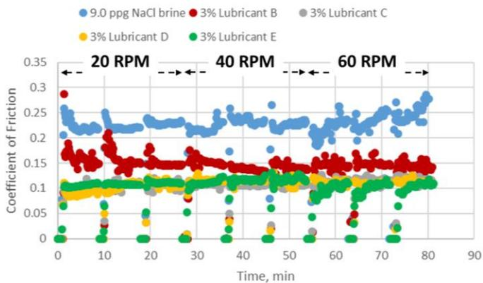
Figure 2: Lubricity of 9.0 ppg NaCl brine on steel-shale contact measured with the dynamic lubricity tester.
