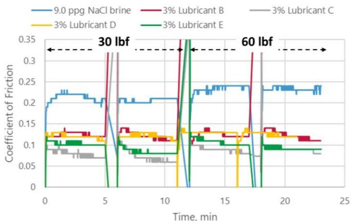
Figure 4: Lubricity of 9 ppg NaCl brine on steel-shale contact measured with the LEM.
