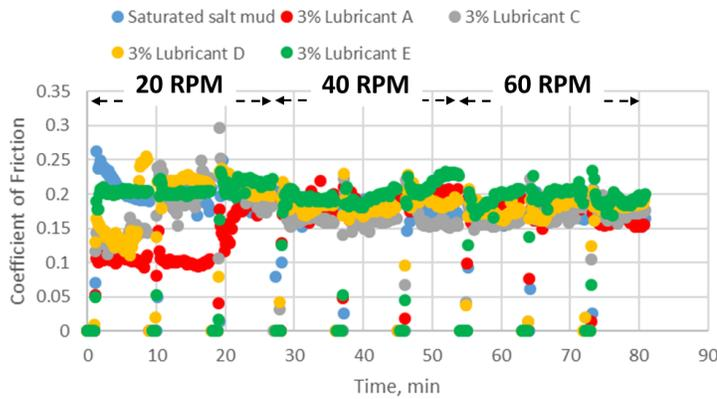
Figure 5: Lubricity of 14.0 ppg saturated salt mud on steel-steel contact measured with the dynamic lubricity tester.
