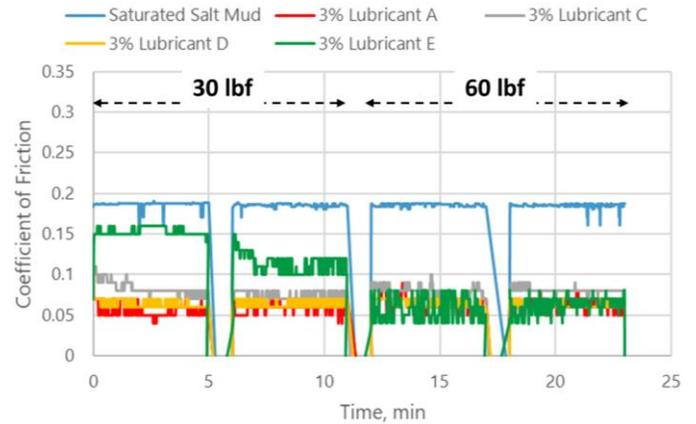
Figure 8: Lubricity of 14.0 ppg saturated salt mud on steel-shale contact measured with the LEM.
